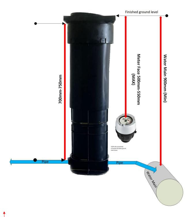
Meter face from GL - 500mm (min) and 550mm (Max)
